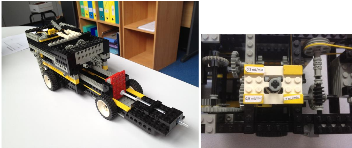
Figure 2. “Home-made” micro-injector. Four rates of injection are available (zoom on the gearbox).
